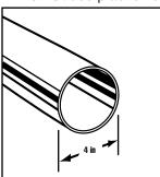
Use 4-inch heavy metal or flexible metal vent. Do not kink or crush flexible metal vent. It must be completely extended to allow adequate exhaust air to flow. Check vent after installation. Refer to your Installation Instructions for proper length requirements of vent.
